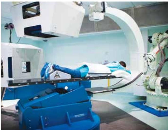
*CNAO treatment room equipped with a C-arm custom robotic device integrating x-rays and cone beam CT. (CNAO)*
