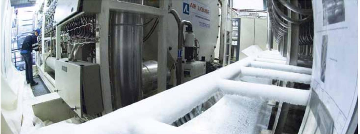
*The cooling and operation of superconducting RF cavities and magnet systems for particle accelerators and magnets for detectors requires large quantities of cryogenic fluids. (CERN-EX-0606020-01)*
