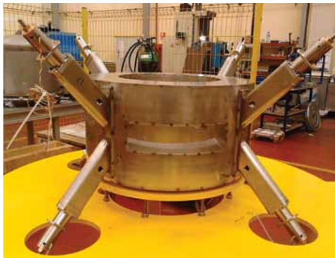
*Components of the AMIT mini-cyclotron. (CIEMAT)*
