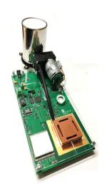
Prototype of the innovative radon monitoring device RaDoM.
